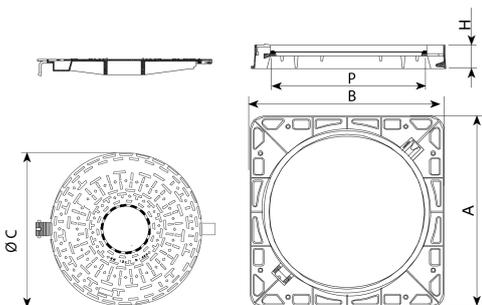
Hexa Max is designed to support medium soft. It is perfect for installing on roads with an ADT of 1.000-20.000, particularly road carriageways (including pedestrian streets), stabilised hard shoulders and parking areas for all manner of vehicles.
