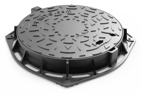
Elyp is designed to support medium traffic. It is perfect for installing on roads with an ADT of 1.000-20.000, particularly road carriageways (including pedestrian streets), stabilised hard shoulders and parking areas for all manner of vehicles.
