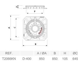
Hexa is designed to support medium traffic. It is perfect for installing on roads with an ADT of 1.000-20.000, particularly road carriageways (including pedestrian streets), stabilised hard shoulders and parking areas for all manner of vehicles.
