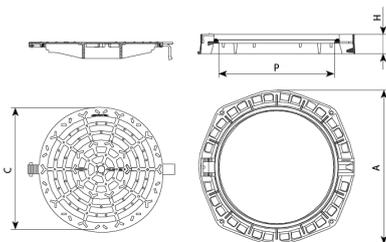
Hexa R is designed to support medium traffic. It is perfect for installing on roads with an ADT of 1.000-20.000, particularly road carriageways (including pedestrian streets), stabilised hard shoulders and parking areas for all manner of vehicles.
