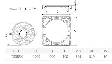
Hexa Max is designed to support medium soft. It is perfect for installing on roads with an ADT of 1.000-20.000, particularly road carriageways (including pedestrian streets), stabilised hard shoulders and parking areas for all manner of vehicles.
