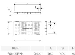
Tango D4 is designed to support heavy traffic. It is perfect for installing on roads with an ADT of 1.000-20.000, particularly road carriageways (including pedestrian streets), stabilised hard shoulders and parking areas for all manner of vehicles.
