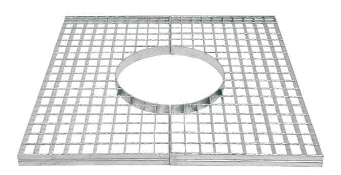
Tree protector made of **34 x 38mm electro-welded mesh**, 30 x 2mm stand brace, 4mm-braid square divider. Finish: hot-dip galvanised. 300mm inner diametre.
