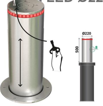
Bollard designed for controlling the access to the public road, communities of neighbours, companies, etc. AISI-304 satin stainless steel piston, Ø220 x 500 mm height. Top lid, chassis, fixing and screws made of stainless steel.
