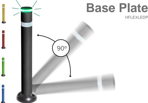
Luminous LED bollard made of flexible black polyurethane resistant to UV rays with reflective band. With base plate for a bolt-on installation. Manufactured in fixed and removable version with polyurethane or stainless steel base. Exceeds a flexion of 1500 cycles at 45° and 50 cycles at 90°, without damage.
